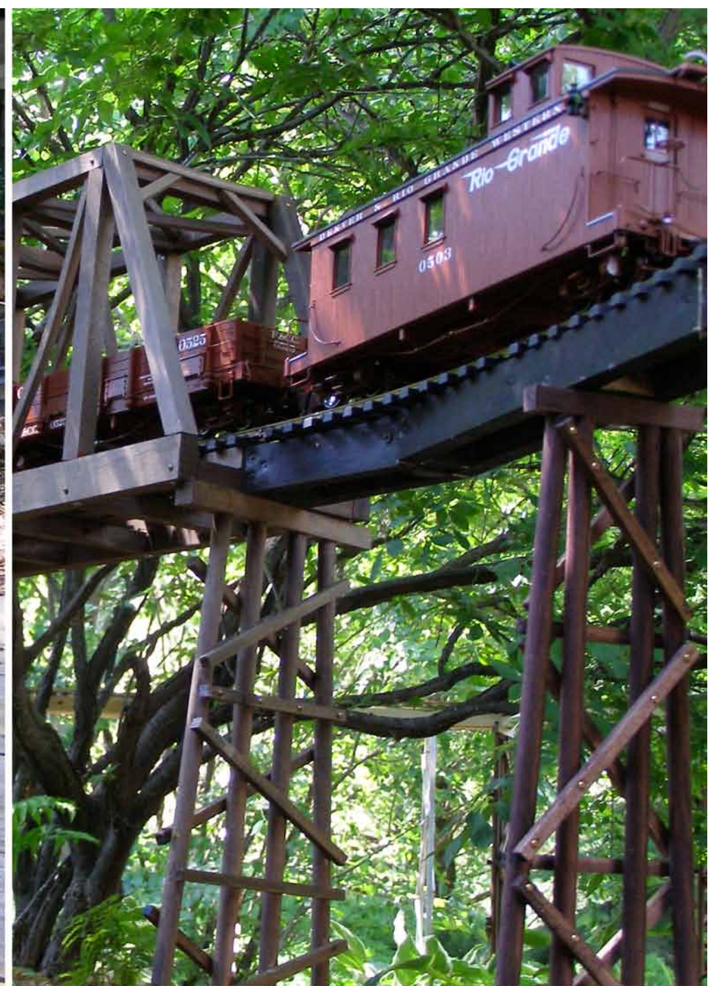
New wooden trestle bents and roadbed deck replaced 2x4 vertical supports and deck planks on the UpperLoop. This improves the appearance as well as making a stronger and stable track support.
